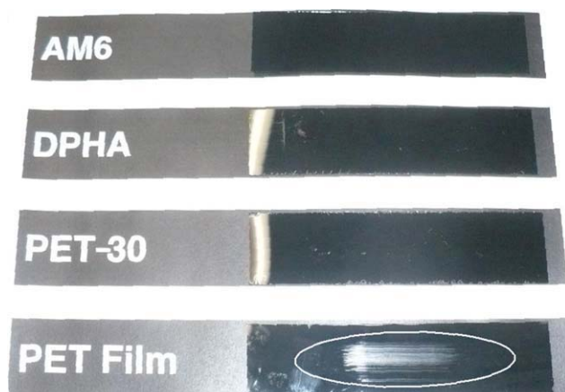
Figure 6 Film photographs of AM6 after scratch resistance test. [Color figure can be viewed in the online issue, which is available at wileyonlinelibrary.com .]
